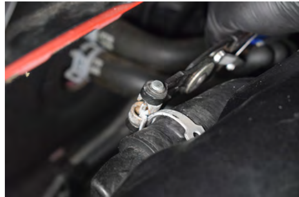
16. Use spring clips to release the clamp.
