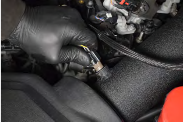
49. Install the temp sensor.
