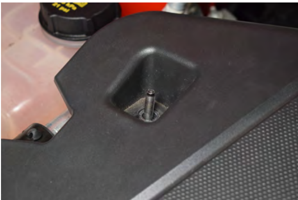
9. Remove the nut on the engine cover.
