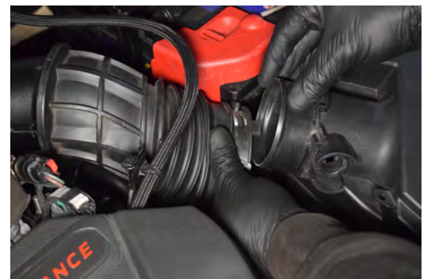
6. The airbox can be removed from the airpipe.
