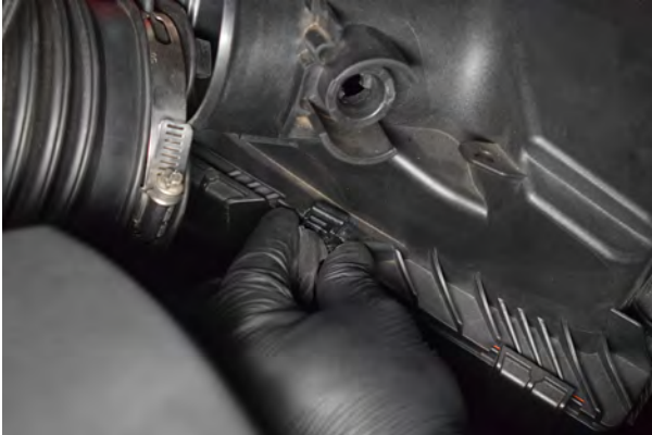
7. As you are removing the airbox remember to unclip the temp sensor wire.
