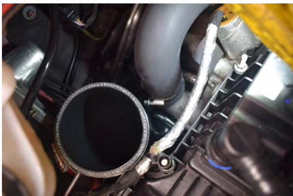
35. Secure the silicone to the turbo with the lower jubilee clamp.
