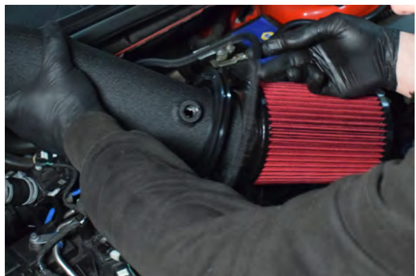
36. You can now position the intake pipe in the engine bay feeding it under the fuel line.
