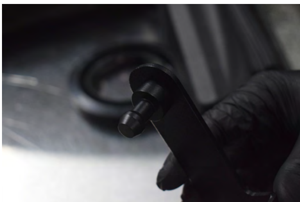
23. Install the supplied bobbins onto the large, folded bracket and secure using supplied bolts and washers.
