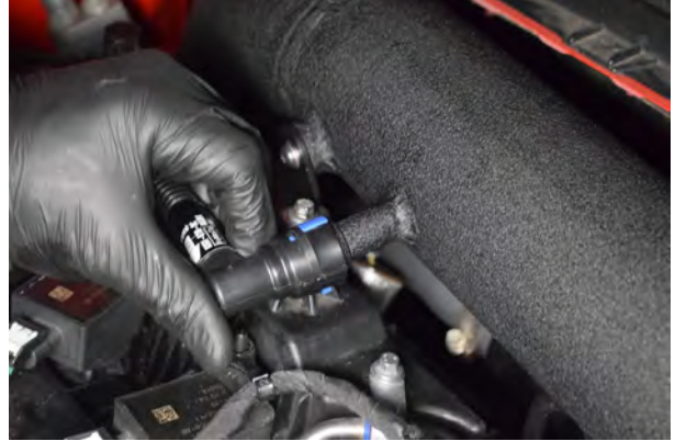
50. Refit the crank case breather, this will click as it is pushed into position.
