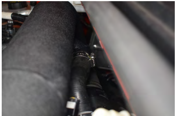
46. Secure using supplied jubilee clamp.
