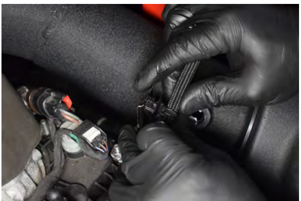
48. Clip the fuel line back into the mounting bracket.
