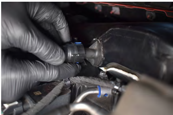
12. Press in the clip on the crankcase breather and remove.
