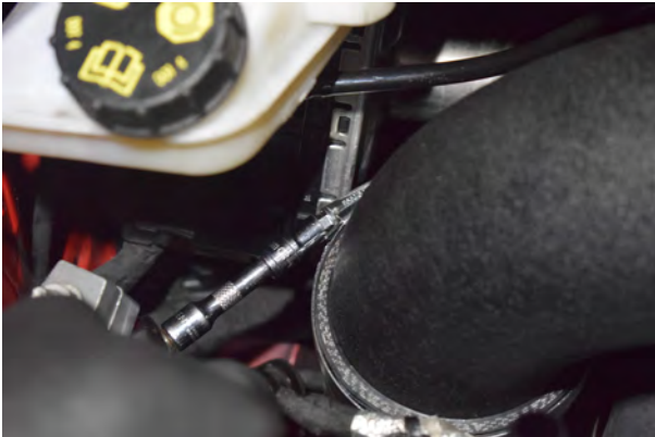
51. Tighten the final jubilee securing the turbo elbow to the intake pipe.
