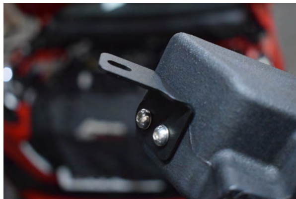
26. The remaining 2x brackets can be fitted to both ends of the wide mouth inlet.
