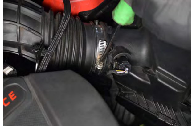
2. Undo the jubilee clamp on the factory airbox.
