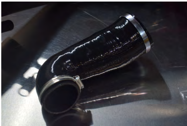
33. Place the jubilee clamps on the silicone turbo elbow.
