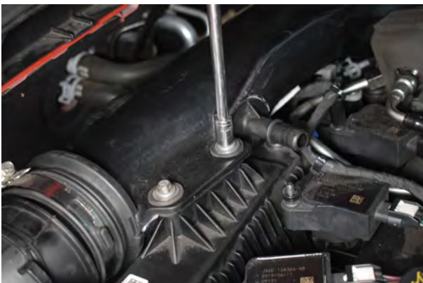
17. Undo 2x bolts securing the air pipe.
