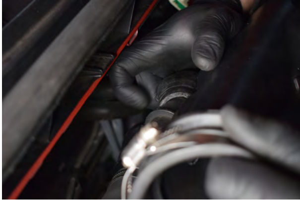
19. As you are removing the air pipe, pull the recirc pipe off.
