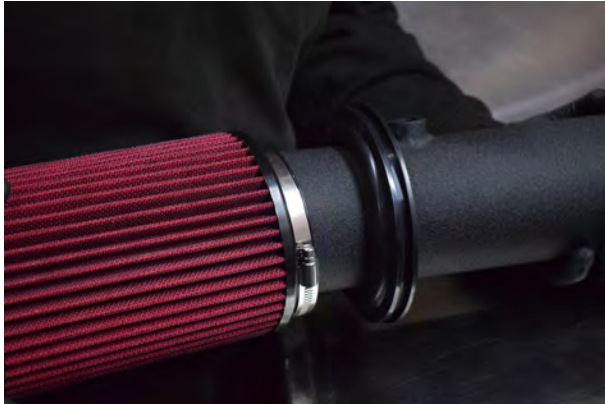
31. Slide the air filter over intake pipe.
