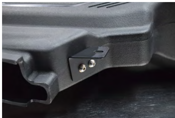
28. Again, use supplied bolts and washers for installation.
