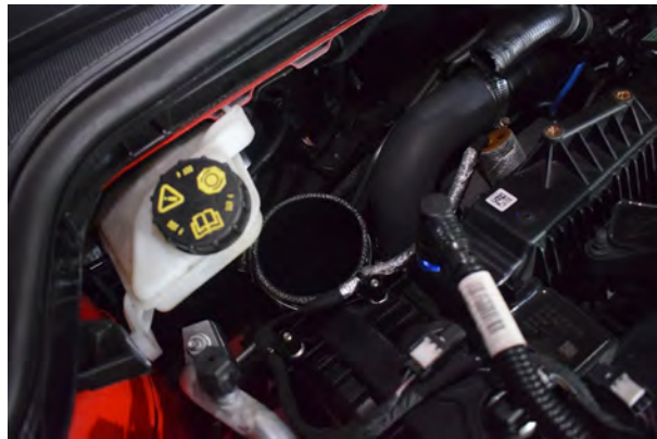
34. Install the turbo elbow onto the turbo.
