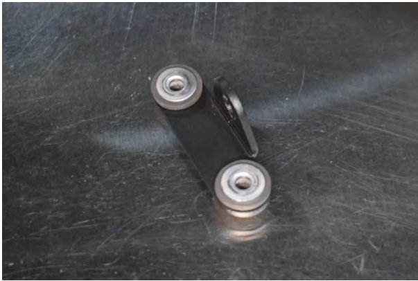
43. Install them onto the Direnza intake bracket.
