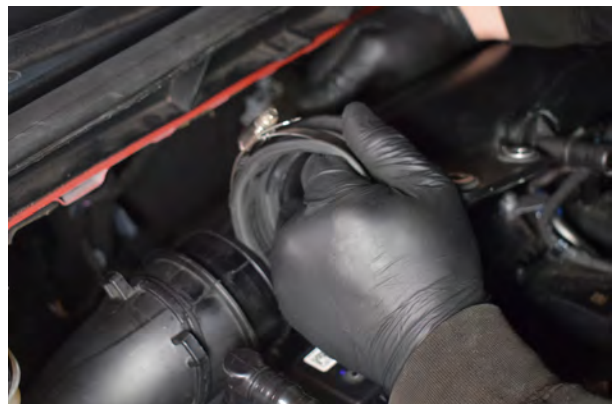
18. The air pipe can now be removed.
