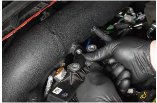
44. Install the bracket onto the intake pipe.
