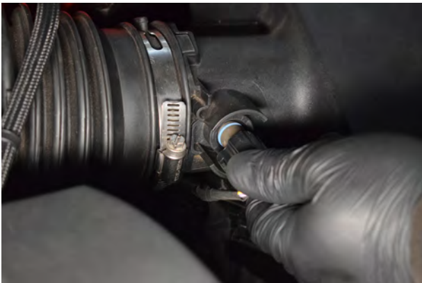
3. Twist & remove the temp sensor.
