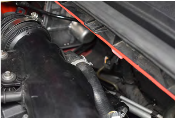
15. The recirc pipe on the rear of the air pipe also needs removing.
