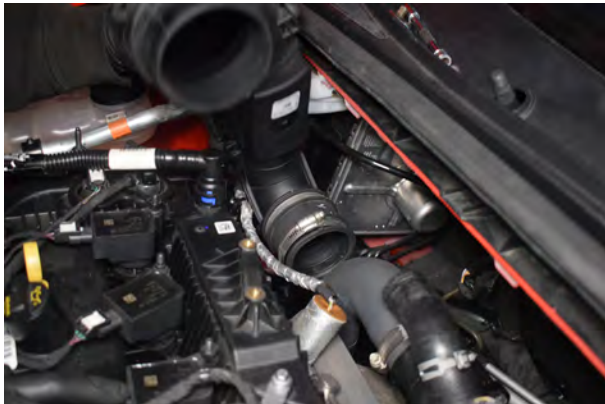
21. The turbo elbow pipe can be removed, by undoing the jubilee clamp securing it to the turbo.
