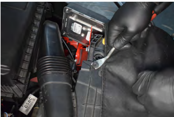
5. Remove the 2x push clips on the front section of the OE panel.
