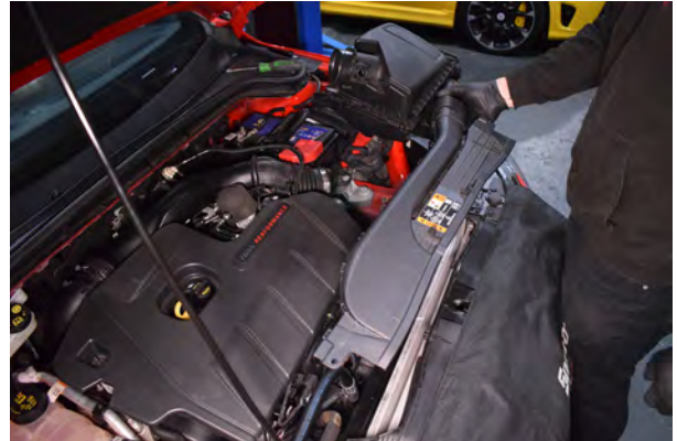
8. The airbox and air scoop can now be removed.
