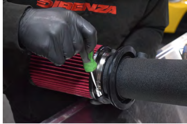
32. Secure the filter with the jubilee clamp.
