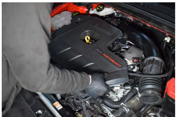
10. Remove the engine cover.
