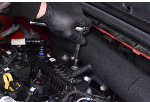
47. With everything in position, the intake pipe bracket can be tightened using the original bolts.
