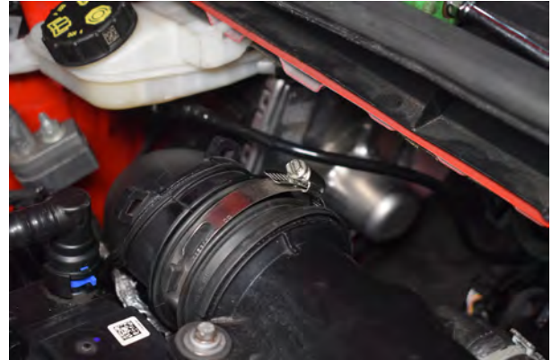
14. Undo the jubilee clamp on the air pipe just before the turbo elbow pipe.
