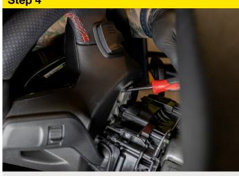
Using a flat head screwdriver, push clips on both sides to release airbag.
