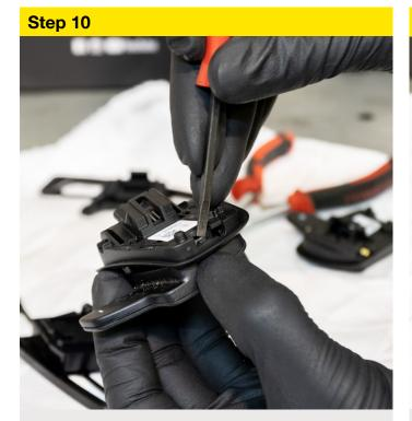
Using flat head screwdriver, push tab in to remove circuit assemblies from OE paddles.
