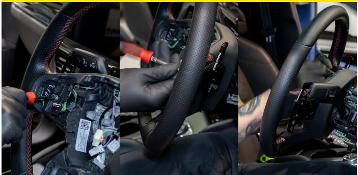
Reattach paddles, fixings and cable connectors
