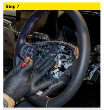
Disconnect paddle cable and remove T27 Torx fixing from both sides.
