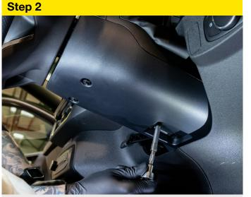
Remove the three, 7mm fixings.
