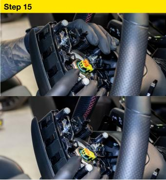
Reconnect air bag, orange connector needs to be pushed in otherwise it won't seat correctly.
