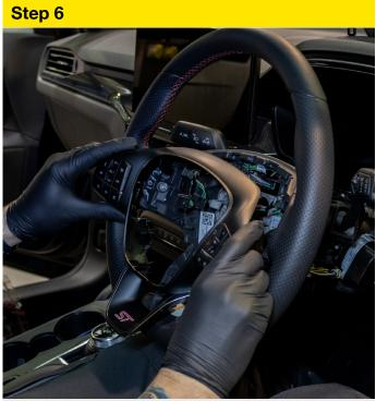
Disconnect cables from buttons and remove trim from steering wheel (gentle force may be required).
