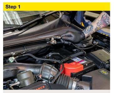
**Disconnect negative terminal from battery** (critical that this is performed first!)
