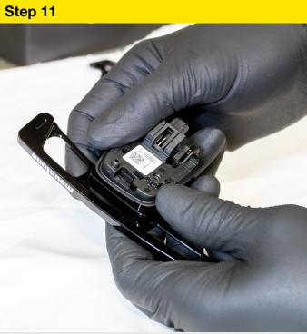
Install circuit assemblies to new paddles, ensuring paddle locks in to tab.
