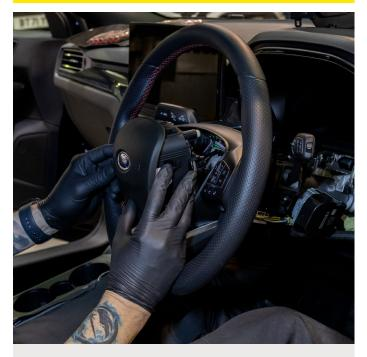
Disconnect cable from airbag and remove - pull orange tab upwards to remove airbag assembly.
