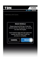
**STEP 3.** When the Tunes screen opens, it will show any vehicles you've worked on. If this is your first time, the list will be empty. Tap READ VEHICLE at the bottom, locate your vehicles OBD port and connect your FLASHlink Device, switch the ignition to the ON position — but don't start the engine.
