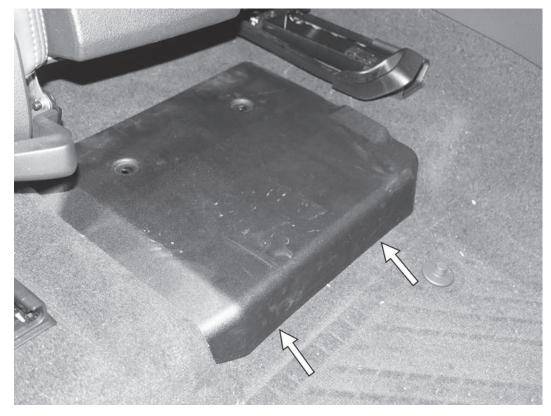
7) Slide the cover back over the electrical connector, ensuring the tabs on the back side of the front of the cover slide back in place on the mounting bracket. Replace the front floor mat if removed.
