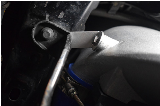
19. Remove 2x bolts from radiator bracket so the intercooler can be installed. At the same time slide the bigger silicone on.
