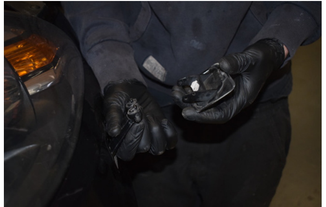
5. Remove the headlight washer jet covers by manually pulling the washers out.
