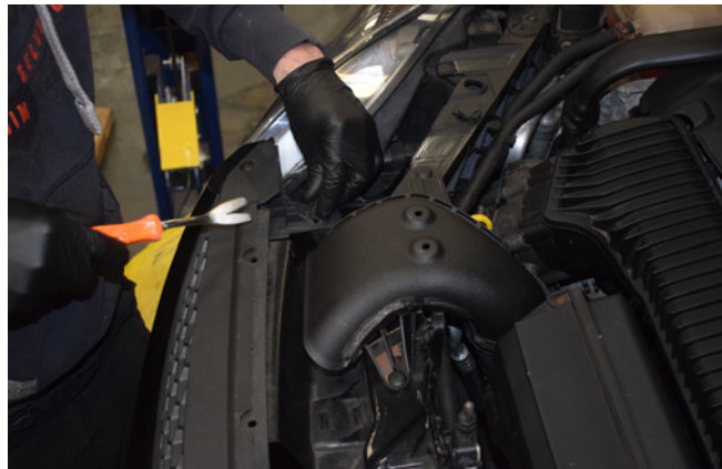
2. Remove the 2x push fittings from the front bumper.
