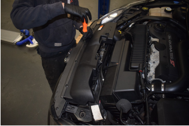
1. Remove the 6x phillips push fit fasteners from the engine bay slam panel.
