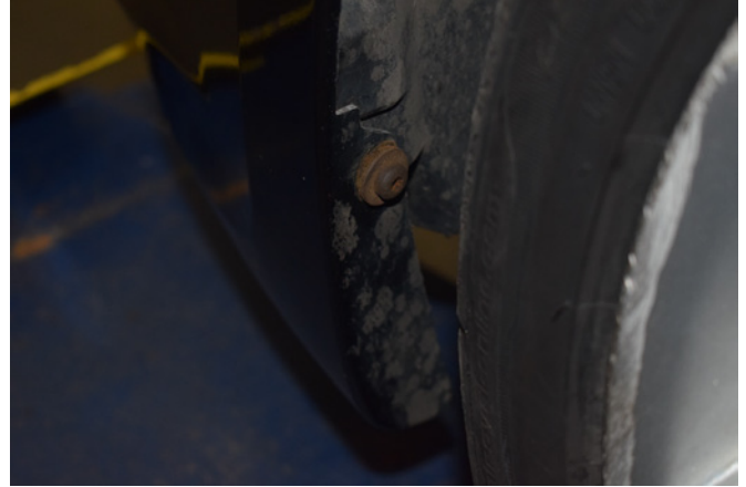
4. Remove the 2x T27 bolts in the outside of the wheel arch.
