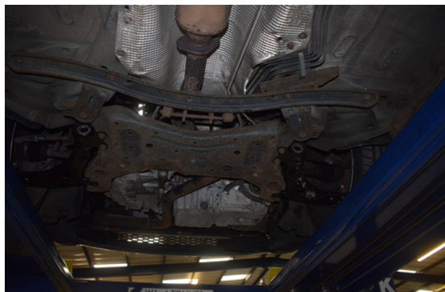
3. Remove the rear undertray and front bumper tray attached with T27 bolts.
