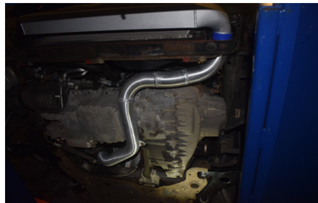
20. Using the short silicone connector and 2 clamps, put the hard pipe back into position - connect to turbo first. Then bolt the pipe to the sump before tightening the clamps.
